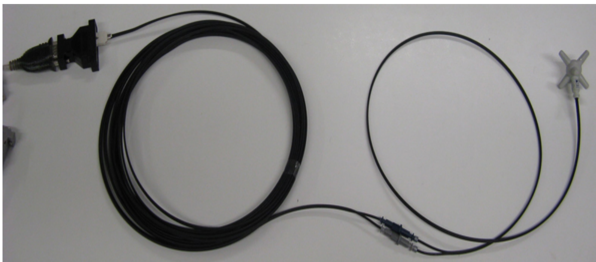
Fig. 2-2 USB connection of EP600/EP601/EP602/EP603 with FO-EP600/10 extension
